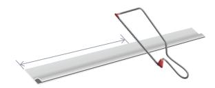
1) Measure the required length and cut the carrier with a fine-tooth saw (or similar).
