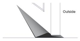
**6) (Optional)** You may choose to install metal fixings (particularly where vehicles will be driving over) to ensure a secure fix.
