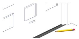
3) Position the floor seal against the INSIDE of the garage door while it is closed, and slide the thinnest part of the seal under the door. Once you are satisfied with the position, use a pencil to mark along the length of the seal. Then, open the door and carefully mark along the outside edge of the seal.
