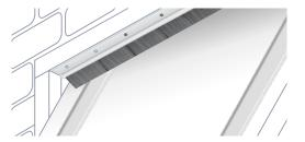
**3)** With the garage door partially open, position the seal where you have marked the frame. Fix using screws, rivets or fasteners at evenly spaced intervals, as required.
