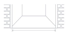
Measure the overall width of the garage door frame from the inside edges. Then cut the seal to the required length by following the cutting instructions provided.
