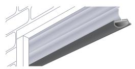
4) Starting from one end, pull back the opposite flap and guide it over the T-bar bottom sections on the roller door. Repeat this process all the way along until completely secured onto the T-bar.
