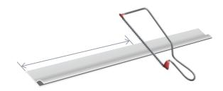
1) Measure the length required and cut the carrier with a fine-tooth saw (or similar)
